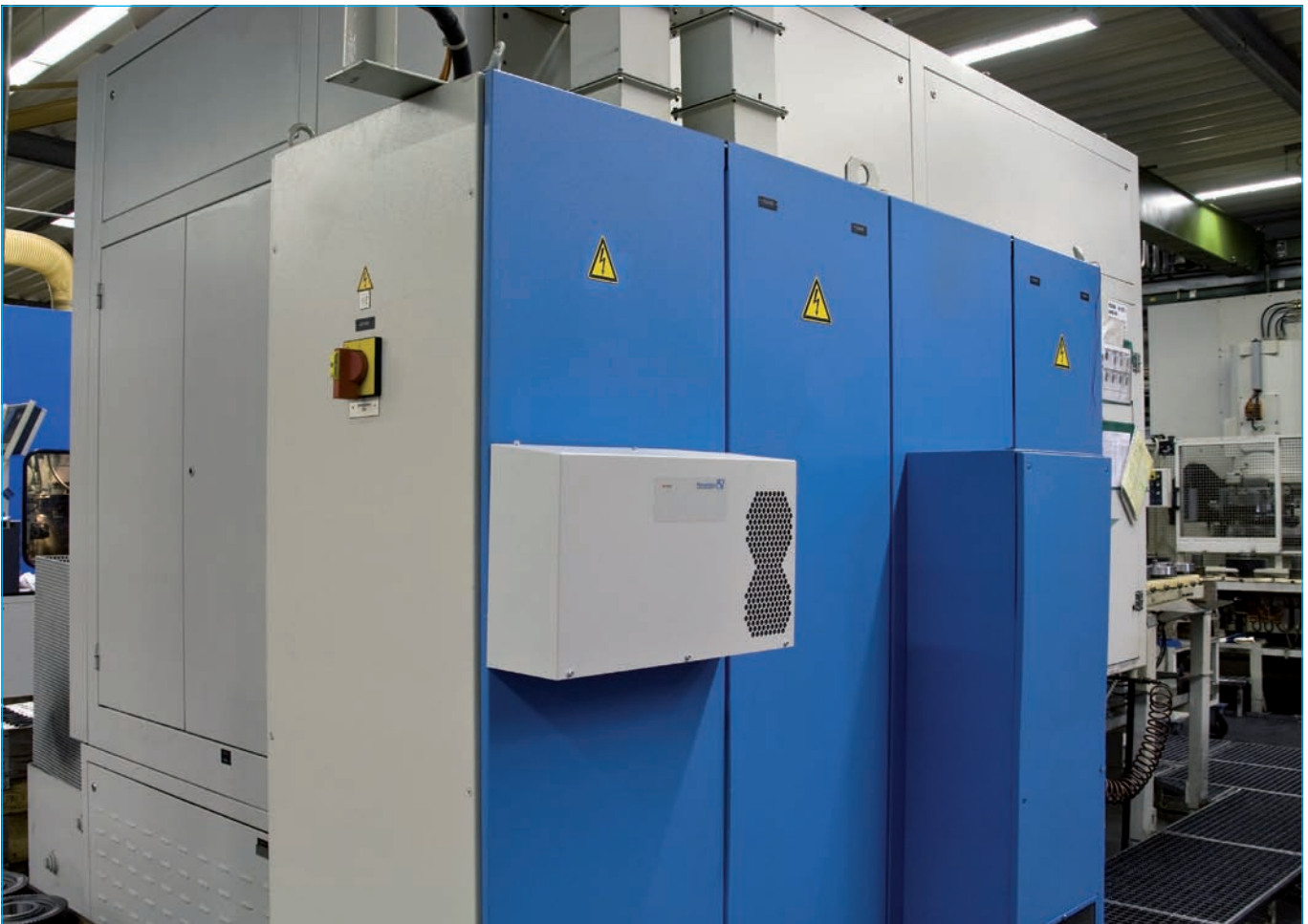
Side mounted cooling units from the Pfannenber DTS series
